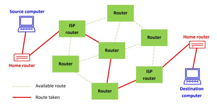
Every computer on the Internet uses a unique set of numbers called an IP (Internet Protocol) address to identify it. Also, the computers all use a common language called TCP/IP to communicate with each other and understand the data being sent (TCP stands for Transmission Control Protocol).
